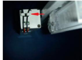
Secure the cables at the motor housing.
