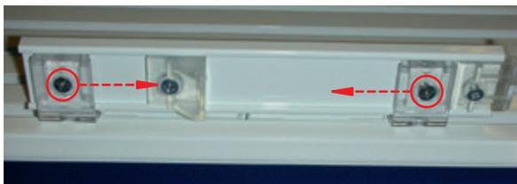
For tensioning the chain you need to reduce the distance between the two runners at the master carrier symmetrically. This will not change the position of the master carrier. End positions will not be affected by this tensioning. The tension has to be checked a second time as soon as the system carries the fabric.
