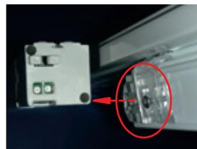
Attach a panel end cap (marked with a red circle) to the master carrier. Then with a sharp nipper, cut off everything that sticks out towards the motor, to avoid any collision.
