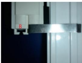
Now attach the motor to the rail with the steel clip. Depending on the rail profile it may be necessary to use the fixing position A (shorter distance) or B (longer distance).
