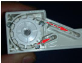
Insert the chain-wheel as shown in the pictures. The wheel will not turn! Therefore, you need to pull at both chain ends to tighten the chain inside the gear. Please add some silicone grease to the movable parts to reduce friction and noise.
