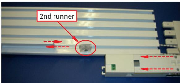
Move the two chain connectors towards each other to pull the chain into the rail. Don't forget to insert the second runner for the master carrier, before attaching the end cap to the rail.
