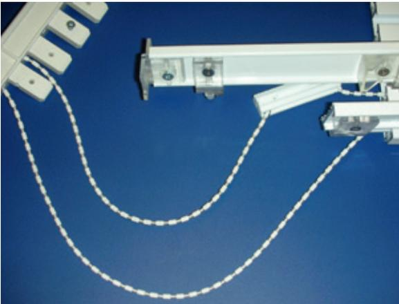
The second master carrier (non drive side) needs to have only one glider between the two runners. If everything was made perfect, the glider will move freely between the two runners until the first master carrier (on the drive side) will start moving the second panel. The drive chain does not need to be cut to attach the glider!
